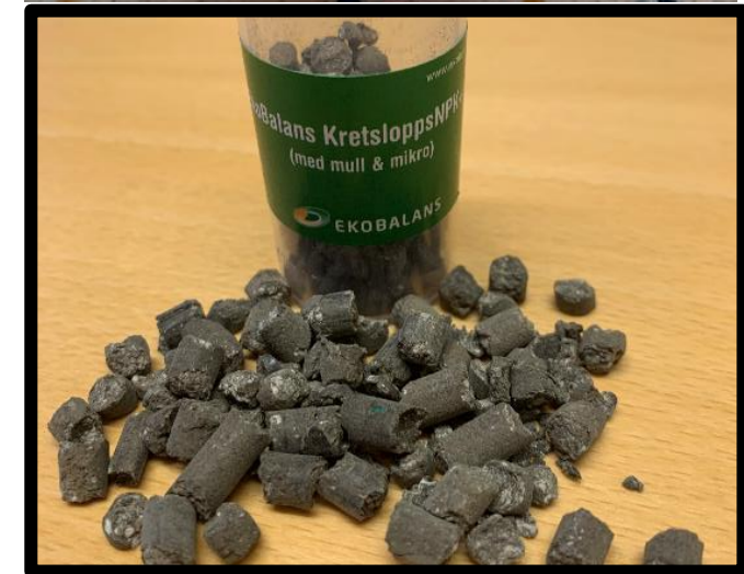
Fertilizer NPK pellet produced from recovered struvite / ammoniumsulphate and digester sludge gave good results in 3 year farm trials***.
